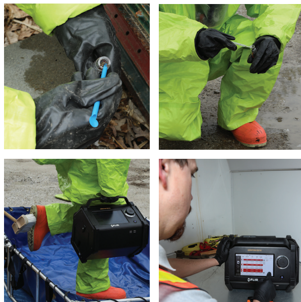
In-Field Sample Collection, Decon, and Chemical Identification with FLIR Griffin G510
